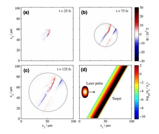
The relativistic energy electron surface current expands at a speed close to the speed of light.
