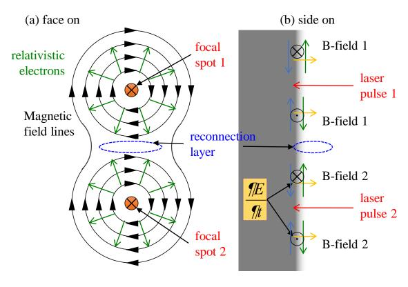
The azimuthal magnetic fields are in the same configuration, but the magnetic field lines are driven together at ~ c
