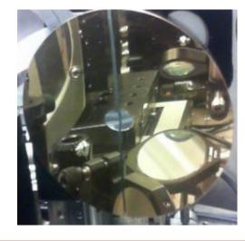
$\lambda = 800 \text{ nm}$ 2 J 40 fs 2 x 10<sup>19</sup> Wcm<sup>-2</sup> Normal angle of incidence OMEGA EP Two separate 20 ps beam lines. Co-timed to +/- 5ps.
