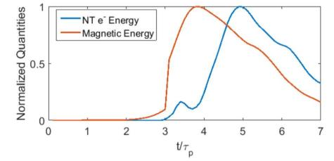
Nonthermal spectral component develops: power law fit  $\frac{dN}{d\gamma} \propto \gamma^{-1.6}$ Consistent with relativistic reconnection Temporal evolution of magnetic potential energy and the energy in nonthermal electrons
